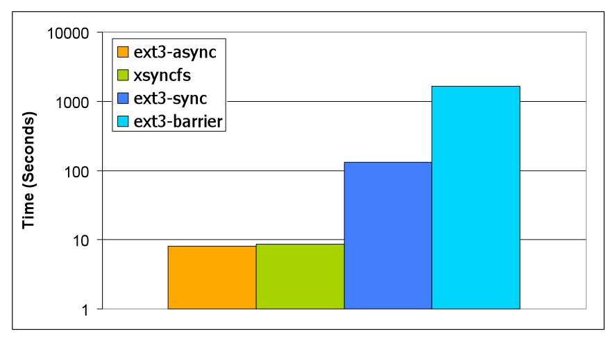
Xsyncfs within 7% of ext3 mounted asynchronously
