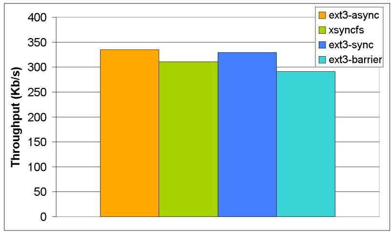
Xsyncfs within 8% of ext3 mounted asynchronously
