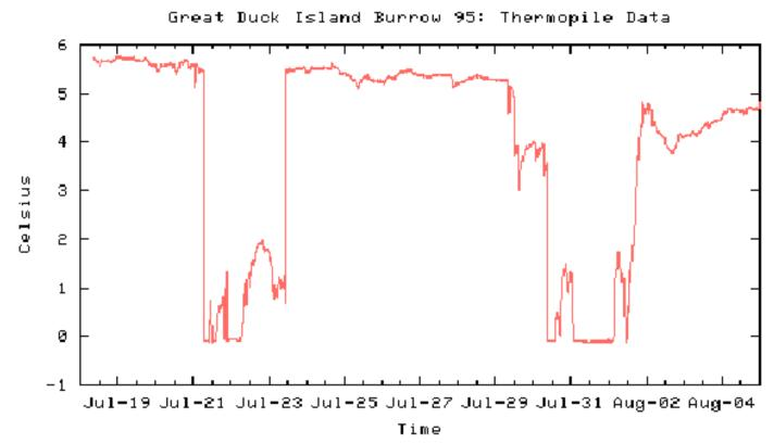
Raw thermopile data from GDI during 19-day period from 7/18-8/5/2002. Show difference between ambient temperature and the object in the thermopile's field of view. It indicates that the petrel left on 7/21, return on 7/23, and between 7/30 and 8/1
