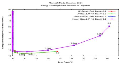
Fig. 4.8 Energy Consumption per KByte of Data Received, Results of History- & Linear Prediction-based Approaches, Microsoft Media Format at 256Kbps
