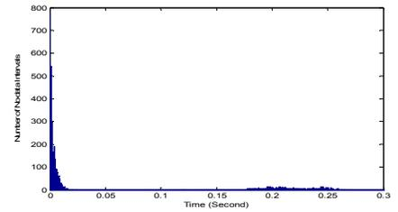
Fig. 4.4(b) No-data Interval Length Histogram for Actual Data, Apple QuickTime Format at 256Kbps
