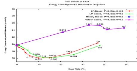
Fig. 4.9 Energy Consumption per KByte of Data Received, Results of History- & Linear Prediction-based Approaches, Real Format at 512Kbps
