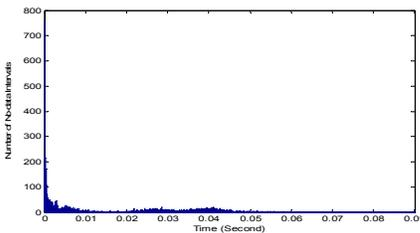
Fig. 4.3(b) No-data Interval Length Histogram for Actual Data, Real Format at 512Kbps
