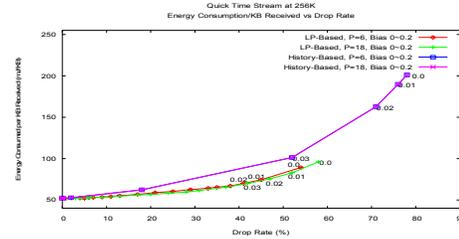
Fig. 4.10 Energy Consumption per KByte of Data Received, Results of History- & Linear Prediction-based Approaches, Apple QuickTime Format at 256Kbps
