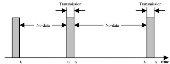
Fig. 2.1 Simplified Stream Packet Transmission in a Wireless Network
