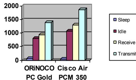
Fig. 1.1 Energy Consumption Rates of Two WNIC's in Various States
