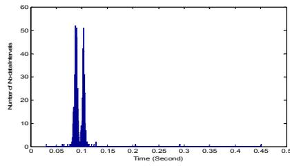
Fig. 4.2(b) No-data Interval Length Histogram for Actual Data, Microsoft Media Format at 256Kbps
