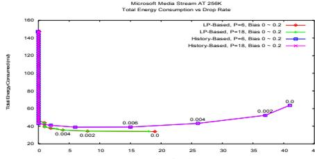
Fig. 4.5 Total WNIC Energy Consumption vs. Drop Rate, Results of the Linear Prediction-based Approach, and History-based Approach, Microsoft Media Format at 256Kbps.
