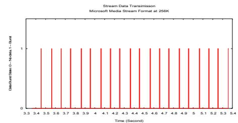
Fig. 4.2(a) Data Burst Intervals for Microsoft Media Streaming Data at 256Kbps
