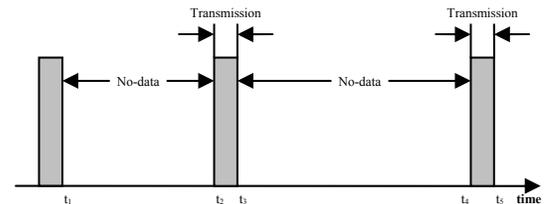
Fig. 2.1 Simplified Stream Packet Transmission in a Wireless Network
