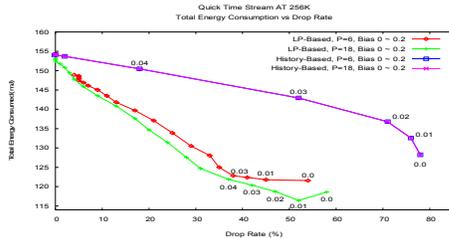
Fig. 4.7 Total WNIC Energy Consumption vs. Drop Rate, Results of the Linear Prediction-based Approach, and History-based Approach, Apple QuickTime Format at 256Kbps.
