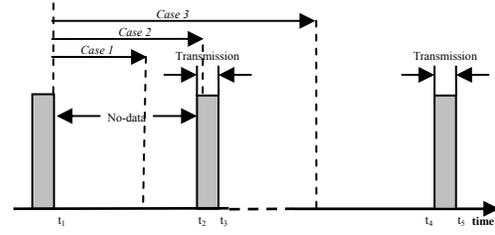
Fig. 4.1 The Predicted No-data Period and the WNIC Energy Consumption Model
